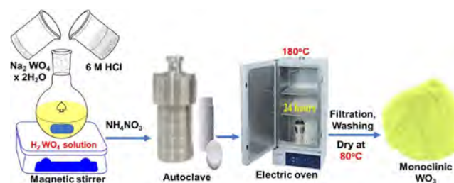
Figure 1. Schematic representation for synthesis of m-WO 3 nanoplates.
